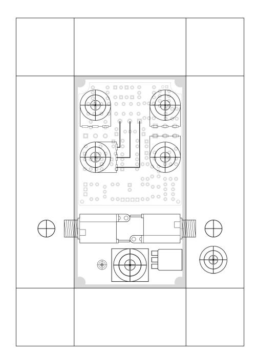
You'll want to use lug pots for all but possibly the volume pot for the 4 knob method, because pc mounts will not line up correctly. The wires for lugs 1 & 3 on the lower gain pot need to be criss-crossed, or CW will lower the gain instead of the other way around.
