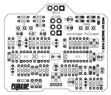
The Flyleaf is based on the vintage EHX Zipper™ Envelope Follower that debuted in 1977. It has been adapted to use true bypass switching and includes an internal trimpot for adjusting the effect for bypass unity via an onboard clean boost. This boost is based on the LPB-1.
