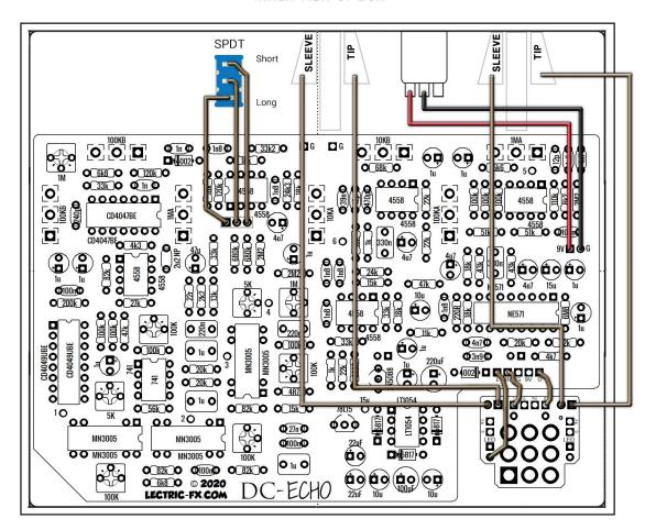
You can twist each of the 2 pairs of wires coming off the mini 3pdt pcb together with a drill if you want, and run them under the pcb up to the tips and sleeves of the in/out jacks, for a very clean look.
