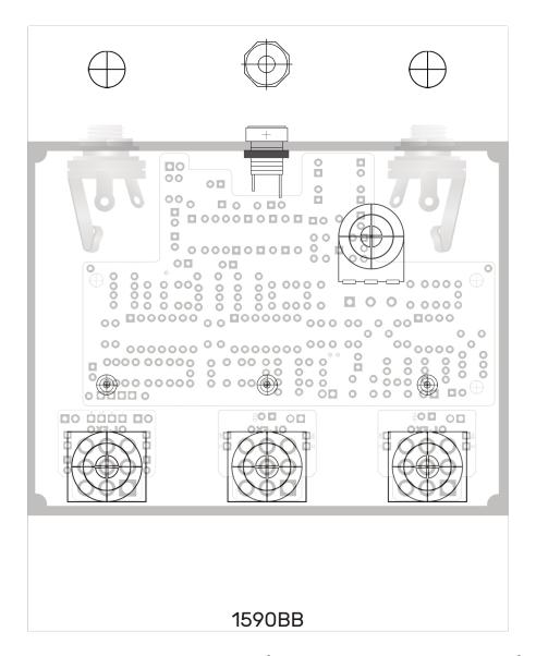
Location for vibe switch mod not shown, as it is left up to the builder. The pot location for the feedback mod is where a pc mounted type would be, but a lug pot can be wired and placed wherever you want it. LED locations are only suggestions, but of course they can be wherever you want as well.
