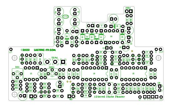
The Altered State is Lectric FX's take on the revered Maestro PS1-A Phaser. Besides shrinking the circuit down enough to fit a 1590BB enclosure, we've also converted it to run from a standard 9V DC supply, while still providing internal +/-12V supply of the original without the need for expensive specialty power bricks. We've also added a few updates for the modern player.
