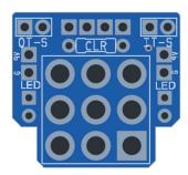
Here's a basic 3PDT breakout pcb we call the "mini" Thripidity. This pcb features a CLR footprint and LED pads on either side for easy placement. 9V & G pads on both sides as well for flexibility regarding DC jack placement. Also includes pads for Input/Output jack Tips/Sleeves.
