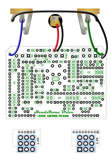
Carefully trim one wire off the provided 10conductor ribbon cable. Then just connect the small pcb's you've soldered to your 2 x 3PDT footswitches straight across to the main pcb with the 6-conductor and 9-conductor cables.
