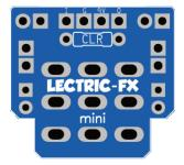
Here's a basic 3PDT breakout pcb we call the "mini" Thripidity. This pcb features a CLR footprint and LED pads on either side for easy placement. 9V & G pads on both sides as well for flexibility regarding DC jack placement. Also includes pads for Input/Output jack Tips/Sleeves.
